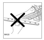
Check that the WRD is not clogged with detergent residue. If necessary rinse it under running water after having removed it
